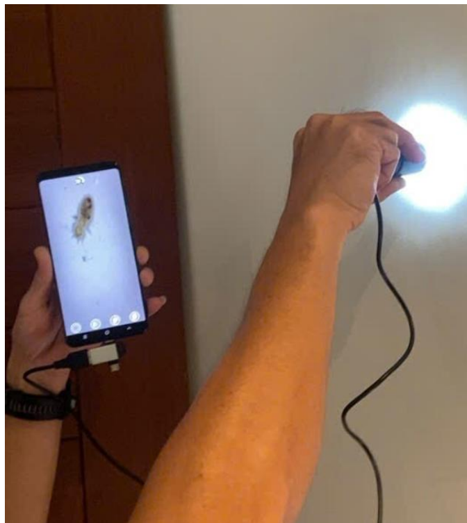
Camera nội soi, soi khe hẹp Endoscopic crevice inspection camera
