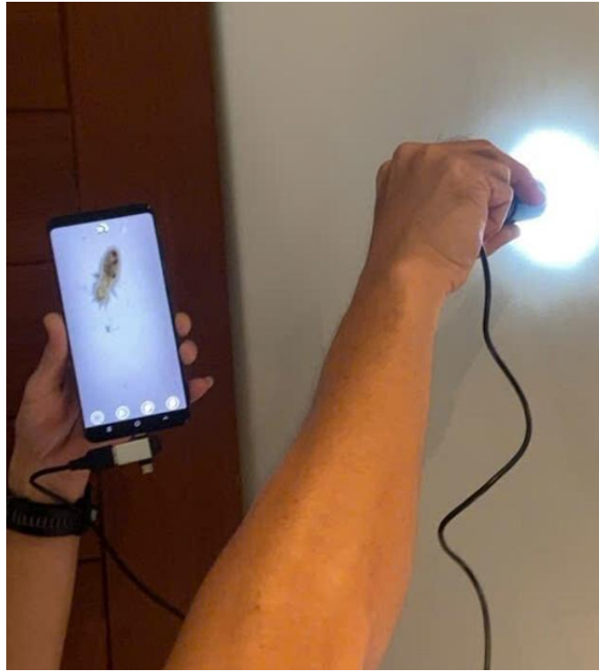
Camera nội soi, soi khe hẹp Endoscope camera for narrow gaps
